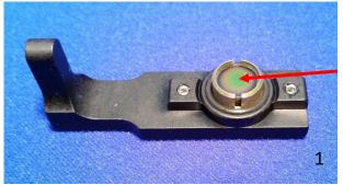
Color Change Indicates FTIR beam focal spot. If the spot is centered in the cup, the PAC300 is aligned.
