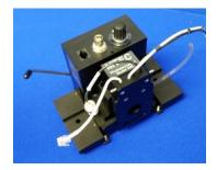
Loosen the top set screw, remove the two top slide plate screws and the attached part which clamps the cables.
